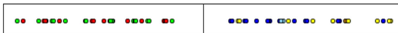
FIG. 2. (Color online) Two examples of clusters exhibited by one-dimensional SO model. The parameter values here are c=1.0 , c_3=1.5 , \alpha=1.5 , N=30 , and L=100 . The initial conditions are such that the positions and the phases are randomly distributed. Color (grayscale) represents the phase of each element. These are final states where all positions and phases of the elements are static. Although these calculations are held with the periodic boundary condition, behavior in this system is the same as what is investigated in this paper because the system size is large enough.
